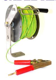
clamped to the side plate. This ensures a clean 100% contact. Because the hub is not required for continuity it is made from rigid PVC which provides a maintenance free bearing. Stainless steel is used for all other major components. A dedicated clip stowage point prevents clip loss and inadvertent unreeling during vehicular movement. The reel is fitted with an adjustable friction brake to eliminate over-run when unreeling.
