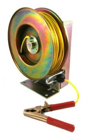
sealed housing, so no water or dirt can affect it's correct operation. The rewind speed is controlled using a Silicone fluid damping system which is inherently reliable, and is unaffected by large temperature variations. It's performance will also not deteriorate due to mechanical wear and tear. In older designs the combination of complex rewind speed control devices with the low spring quality has been the major reason for premature failure when operator abuse takes place.
