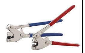
Alpha numeric characters can be engraved onto the dies on request. The characters are then transferred to the seal when it is compressed and identify which set of pliers (and so which operator) carried out the sealing operation.
