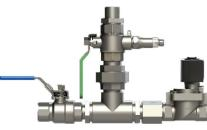
The Faudi aviation DRAINGUARD® is a fully automated drainage system that is fitted in the sumps of Filter Water Separators. It uses the SLUGGUARD® to detect water in the fuel and when the water reaches a predetermined level it sends a signal to the control unit. The control unit in turn sends a signal to the electronic drain valve causing it to open and allow the water to drain through the drain line. Once the water level has
