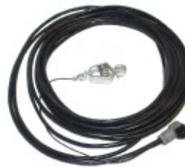
Transducer Cable for test rig
