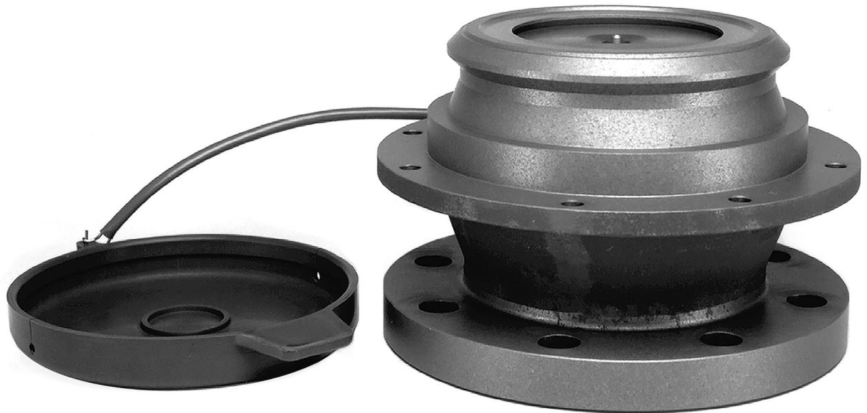
Eaton's Carter 4 inch adapters are made in accordance with API Bulletin 1584 to mate API 1584 compliant hydrant or bottom loading couplers. These adapters are furnished with flanges to mate 4 inch ANSI 150 lb. flat or raised faced flanges. Both ductile iron and aluminum materials are available. These adapters are designed to be used for bottom loading of a refueler, for connection to a hydrant system or for tank farm pumping system for test adapters.
