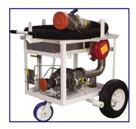
The HC cart is a standard chassis which can be fitted with a range of fluid motors and additive pumps, accessories and additive reservoirs. This allows a complete bespoke system to be supplied in a short leadtime and without incurring the expense of a custom designed system.
