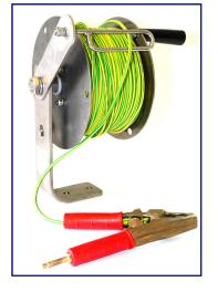
required for continuity it is made from rigid PVC which provides a maintenance free bearing. Stainless steel is used for all other major components. A dedicated clip stowage point prevents clip loss and inadvertent unreeling during vehicular movement. The reel is fitted with an adjustable friction brake to eliminate over-run when unreeling.
