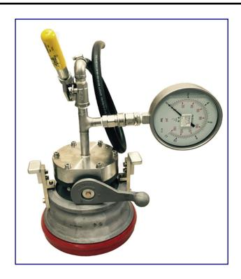
fuel to drain safely into the hydrant pit or a bucket and a calibrated pressure gauge mounted on a tee piece. The gauge is connected via a dry disconnect to allow easy removal for re-calibration or safe storage.
