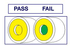
This is a Go/No Go test, the result should be either Pass or Fail as shown above. It should not be used in an attempt to quantify water levels but a slight intermediate colour change can indicate a trace of water in the product somewhere between 0 and 30ppm, and this is shown in the records as Trace if required by local regulations.
