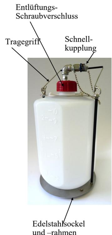
**Gammon Mini Monitor / Multi Mini Monitor Kontaminations –Testkit**
