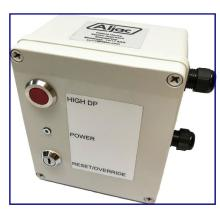
**Deadman Warning Lamp Output.** Lamp 'On' when the Deadman System is activated. Flashes during the Time Out period when system reactivation is required.
