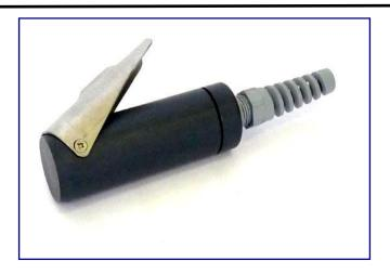
Cable termination is inside the body and uses a two way screwed terminal block, and we can supply the handswitch either with or without cable fitted. The free end of the cable can be terminated in your own junction box or with a weatherproof Niphan 2 pin Plug and Socket. A full range of operating spares is also available from stock.
