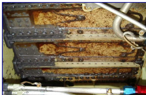
Microbial growth in an aircraft fuel tank
